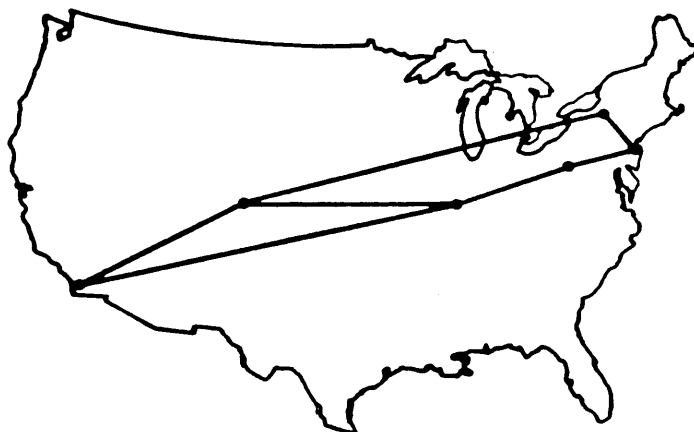
Fig. 5. Planned backbone network connecting NSF-sponsored supercomputers at Cornell University, the John von Neuman Center, at the University of Pittsburgh, the University of Illinois, the National Center for Atmospheric Research, and the San Diego Supercomputer Center. The links will be 56-kbps terrestrial digital circuits connecting network gateways at each site. The supercomputer front-end computers will run the NSFnet standard protocols (TCP-IP and associated application protocols). The NSFnet backbone network will be connected to the ARPANET, to various regional and state networks, and to the planned NSF supercomputer center networks to provide NSF-sponsored supercomputer users with access to all the NSF supercomputer centers. [Courtesy of the NSF's Office of Advanced Scientific Computing]
