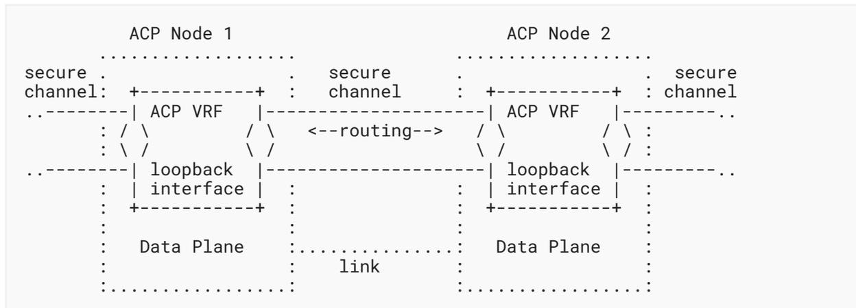
Figure 1: ACP VRF and Secure Channels
